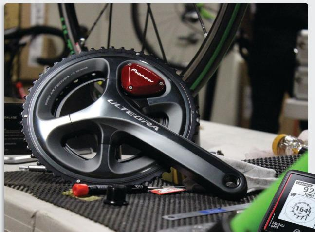
data every 30-degrees of rotation and transmits this wirelessly to the head unit. Currently, it is only available as a Shimano Dura Ace or Ultegra system. It holds a +/- 2-percent accuracy, is highly water resistant and the batteries are user replaceable. The Dura Ace model weighs 700 grams, which is less than both SRM and Quarq units.
